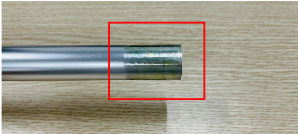
Picture 3: Apply glue to outer tube
