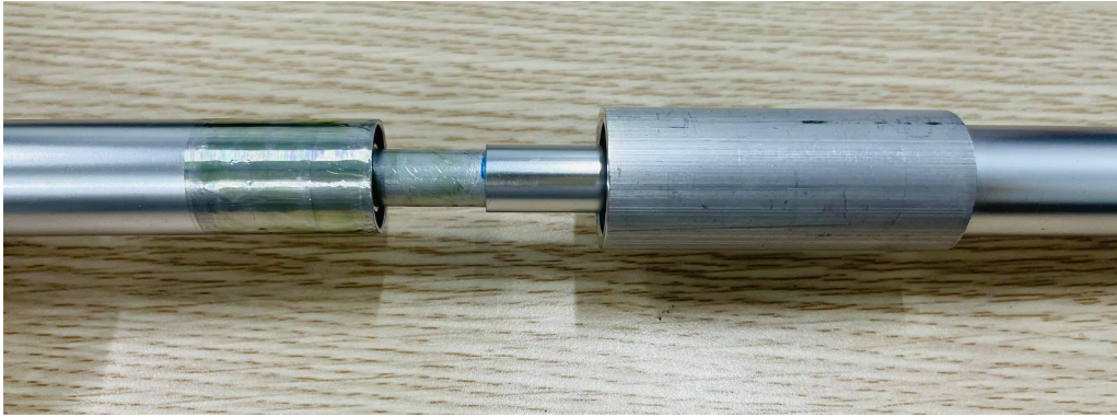
Picture 4: Installing the tube extender to sensor tube
