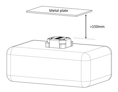
**Notes**: Ensure a minimum clearance of 200 mm between the top of the sensor and any overhead metal surface.
