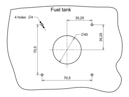
Notes: The mounting hole diameter depends on the material and thickness of the tank
