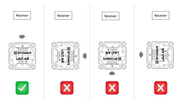
**Notes**: Install the sensor in the direction of maximum signal transmission (the directional arrow on the sensor cover should point toward the receiving device).
