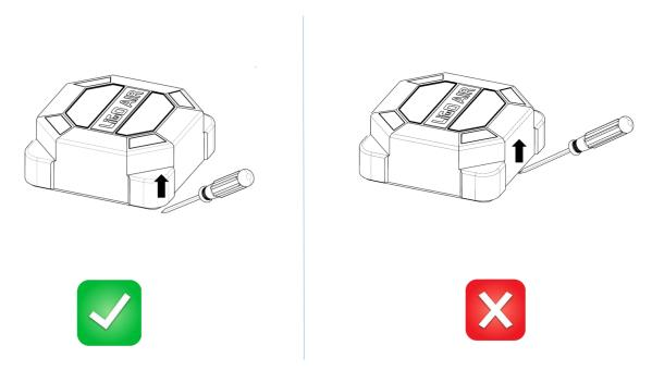
**Notes**: Please ensure that no parts of the sensor are damaged while removing the protective cap.
