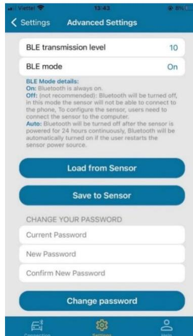
**BLE transmission level:** This option allows users to set the transmission intensity for the sensor (from 0 to 10).
