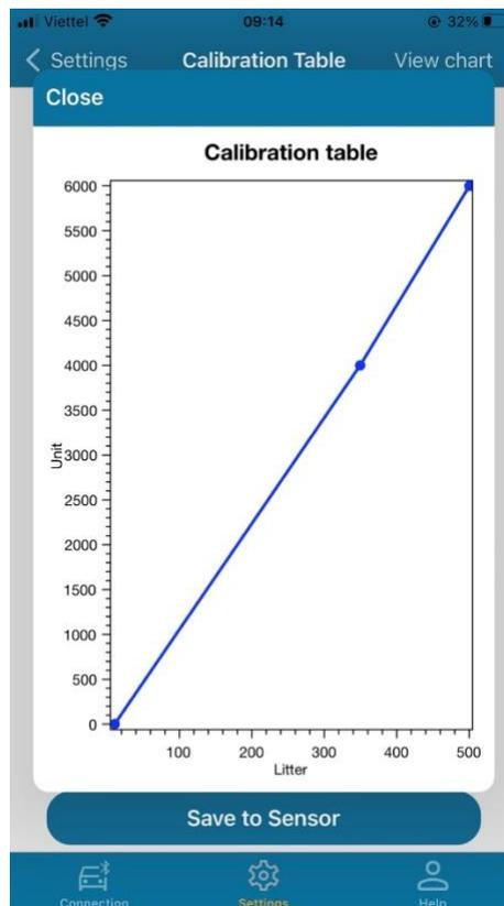
The Calibration chart can show if the calibration process is being done correctly. The graph will be a figure moving upwards from left to right; if any abnormal points are observed on the graph (*The subsequent value of 'Litter' is smaller than the previous value*), users must check to ensure the calibration is being conducted accurately.
