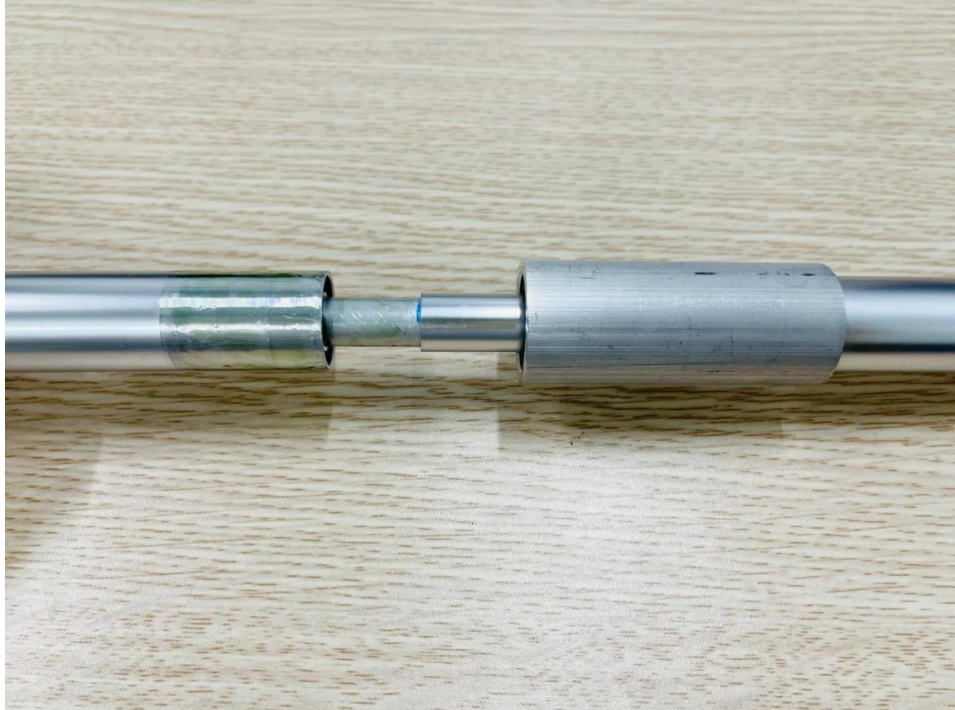
Picture 4: Installing the extender tube to sensor
